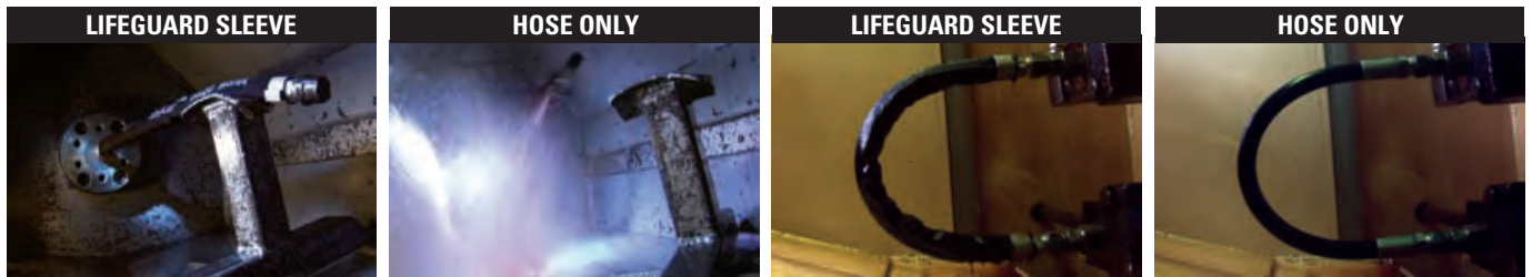
The LifeGuard™ sleeve contained and effectively redirected fluid during 10,000 psi (68.9 MPa) burst tests while hoses without sleeving exploded, releasing a large amount of fluid in the immediate area.
